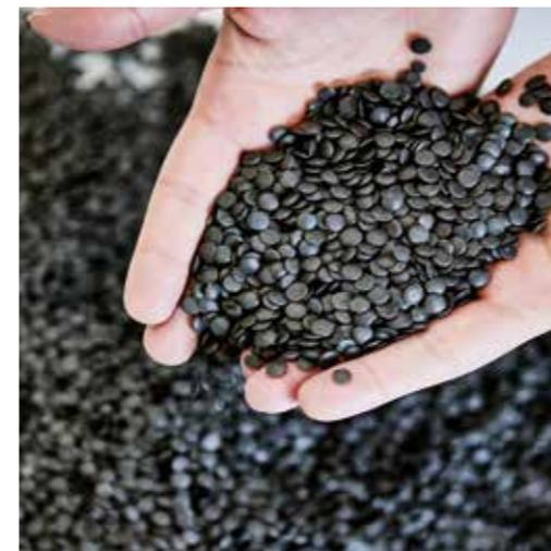
Longer-lasting sustainable road paving thanks to the use of thermoplastic polymers from innovative recycling processes.
